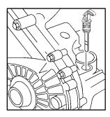
1. The manual transaxle dipstick is located below the brake master cylinder, near the rear of the transaxle case. Flip the handle up and then pull out the dipstick and clean it with a rag or paper towel.
